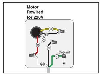
Figure 5. Motor rewired for 220V.
